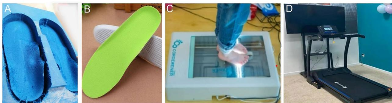
**Fig. 1** Images of Insoles and Measurement Equipment. **A.** Custom accessory navicular corrective insole **B.** Standard insole **C.** CORDEWENAR foot scanner **D.** Treadmill-based foot pressure testing system
