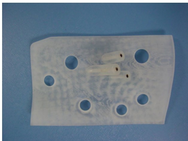
Fig. 5 Input the designed guide plate in STL format into the 3D printer to print the actual guide plate
